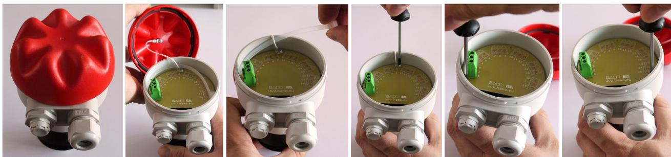
2. Feed the sensor cable from below into the connection head through the cable gland
