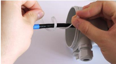
Double wrap cable tie around the sensor cable
