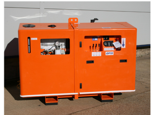
Vikoskim can be powered by a powerpack or by ships hydraulics
