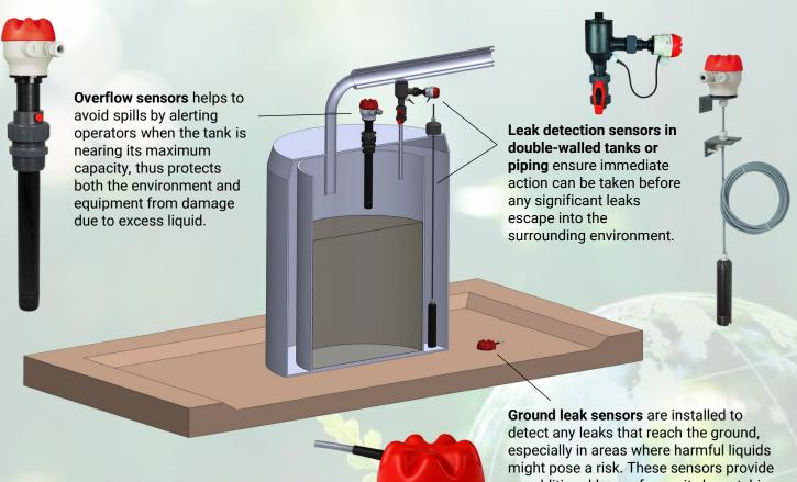
an additional layer of security by catching leaks that may go unnoticed until they reach critical levels.
